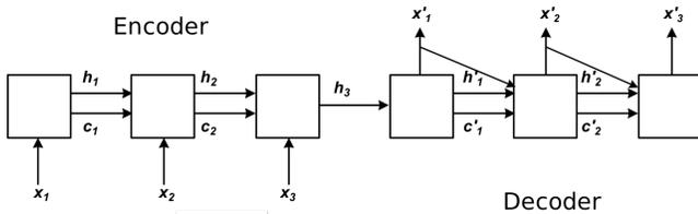
Figure 2: The LSTM Autoencoder network architecture learns to generate the input token in the decoding phase. Once trained, the encoder can be used to output a vector representation for the text of a query.
