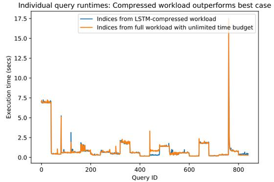
(b) Runtime for each query under our LSTM-based pre-compression scheme and the “optimal” indices recommended by SQL Server. The pre-compressed workload achieves essentially identical performance but with significantly smaller time budgets.
