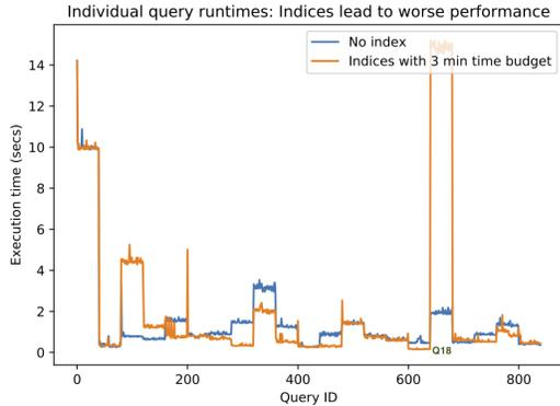
(a) Runtime for each query under no indices and under indices recommended with a three-minute time budget. For a few specific queries (all instances of TPC-H Query 18), the presence of a recommended index results in significantly worse performance.
