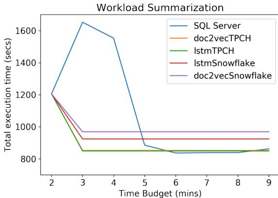
Figure 4: Workload runtime using indices recommended under various time budgets. For most time budgets, the workload summaries improve runtimes, even when the embeddings were trained on an unrelated workload (lstmSnowflake and doc2vecSnowflake).
