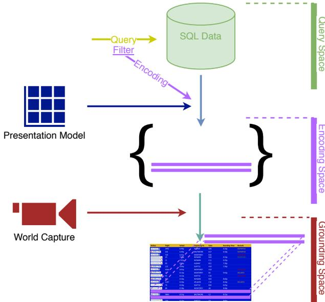
**Figure 3: An overview of the data model used by ARQuery, where multiple result spaces are used to visually encode result sets in AR.**
