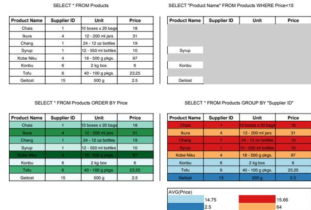
Figure 4: Query operations in ARQuery. Tapping and holding a value filters all rows that contain that value, excluding all others using a visual mask (selection). Tapping and holding a column header excludes the column (projection). Swiping up or down on a column header sorts the column, yielding a sequential color gradient. Swiping right on a column header performs an aggregation, yielding a divergent color annotation and a virtual result pane.
