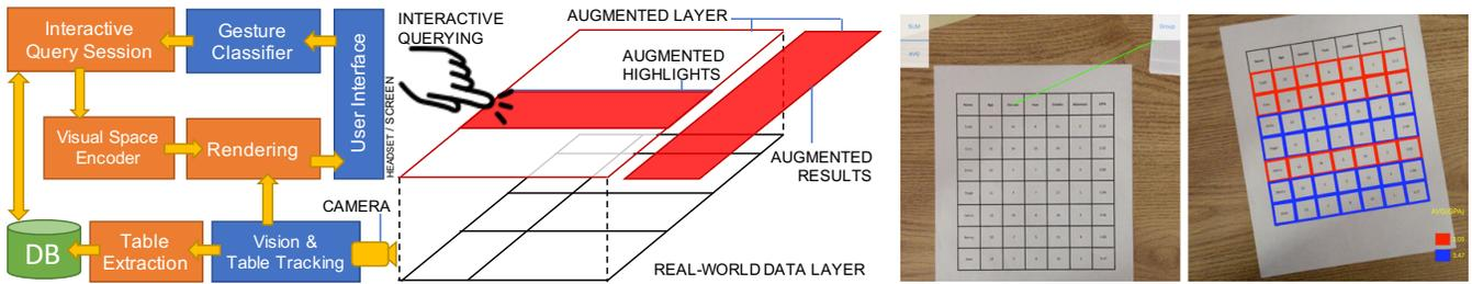
Figure 1: Overall architecture and layers of ARQuery. In this query, a GROUP BY aggregation is performed on a sheet of paper by swiping right on an attribute, yielding a divergent color coding highlights to represent groups, and the aggregates presented as an augmented result legend in the bottom right.
