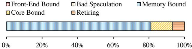
Figure 3: Microarchitectural analysis of SHJ-B on CPU.
